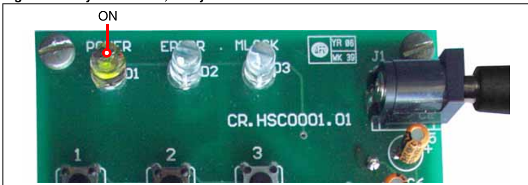
Figure 10. System stable, ready to use
